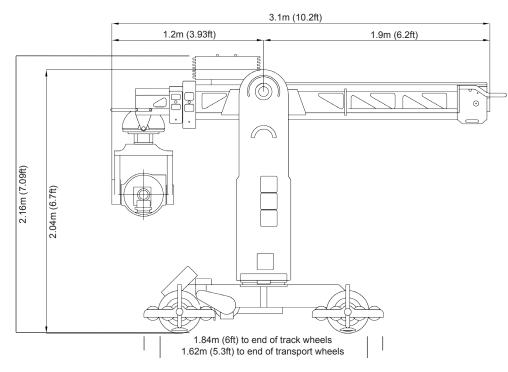
Specifications and Dimensions based on TechnoDolly 15 from Sandstorm Films Serial number 426 with the S head fitted. Measurements based upon safe operation of the crane with the latest software for reliable repeatability at June 2022.
